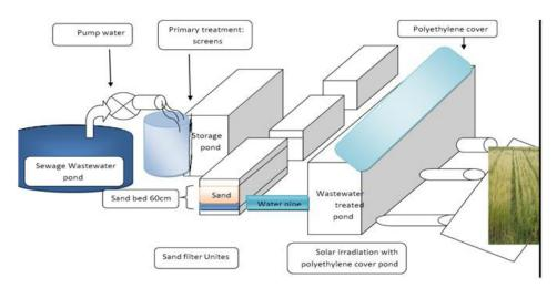
Figure 1. Diagram schematic of sand filter pond and plastic polyethylene cover treatment system
