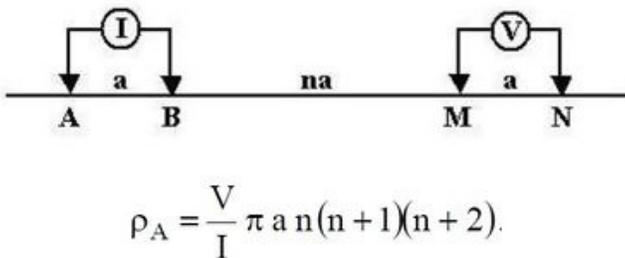
Figure 2 Dipole-Dipole configuration and apparent resistivity
