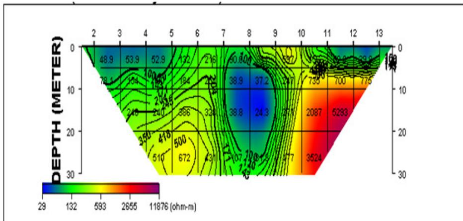
Figure 7 Resistivity Structure along Profile 4
